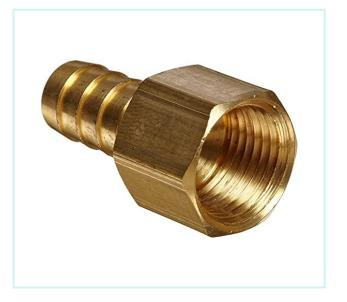
A hose barb is defined as one or more continuous ridger or bumps on a fitting that are used to grip the inside diameter of a tube and seal the connection. As a tube is installed on the fitting, it expands over the barb. grip and seal occur as the tube tries to relax to its original inside diameter behind the barb.
