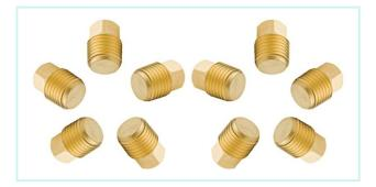
The head plug pipe fitting is made of brass and has a male National Pipe Taper (NPT) threaded connection. this solid square head plug fitting inserts into a pipe or fitting to close and terminate its end and has a square head for an increased bearing surface when adjusting with a wrench.
