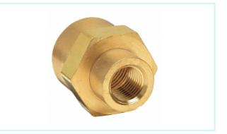
A reducing coupling is designed to accept pipes into either end. For Example a 15mm to 10mm reducing coupling accepts a 15mm pipe into one end and 10mm pipe into the other. A 15mm to 10mm fitting reducer accepts a 10mm pipe into one end and the other end goes inside a 15mm fitting such as an below or coupling.
