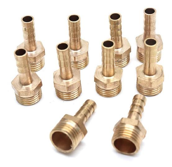
A hose barb is defined as one or more continuous ridger or bumps on a fitting that are used to grip the inside diameter of a tube and seal the connection. As a tube is installed on the fitting, it expands over the barb. grip and seal occur as the tube tries to relax to its original inside diameter behind the barb.
