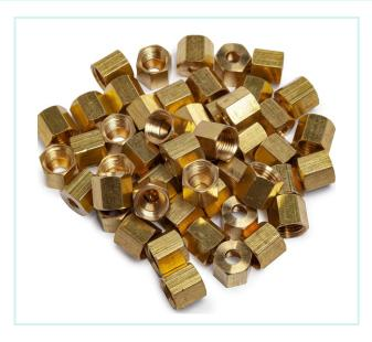
A Compression fittig is a type of coupling used to connect two pipes or a pipe to a fixture or valve.....as the nut is tightened, the compression ring is pressed into the seat, causing it to compress against the pipe and the compression nut, providing a watertight connection.
