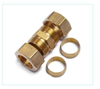
Compression fittings work best when tightened once and not disturbed....this connector is directly placed over the pipe and the nut is tightened compressing the ferrule between the pipe and the body of the fitting. compression of this ferrule also result in deformation of the copper tubing.
