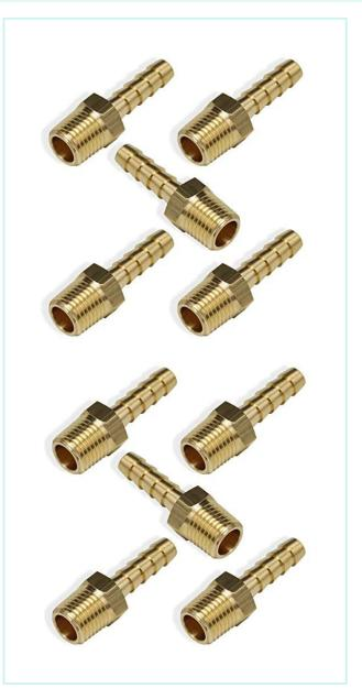
A hose barb is defined as one or more continuous ridger or bumps on a fitting that are used to grip the inside diameter of a tube and seal the connection. As a tube is installed on the fitting, it expands over the barb. grip and seal occur as the tube tries to relax to its original inside diameter behind the barb.
