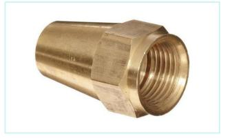
Flare fittings are suitable for use in the plumbing and heating industries for gas, oil, air, and water. they are applicable with brass, tubing, flare fittings can be disassembled and reassembled many times with no effect on the seal.
